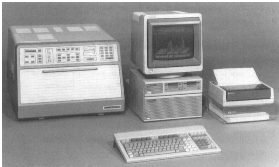
Figure 8. Computer controlled TLC evaluation system which consists of Camag TLC scanner II and Hewlett-Packard Model 310 desktop computer printer.
